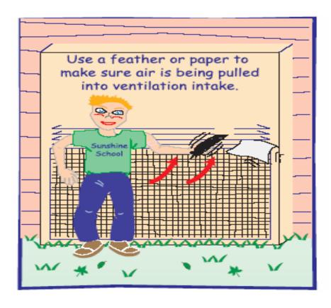
The American Society of Heating, Refrigeration & Air Conditioning Engineers (ASHRAE) recommends that ventilation systems supply 15 cubic feet of outside air per minute per person, constantly while the room is occupied. Many states have adopted this recommendation into their ventilation codes. It takes special equipment to measure air flow, but at least we can make sure that air is being drawn in.
